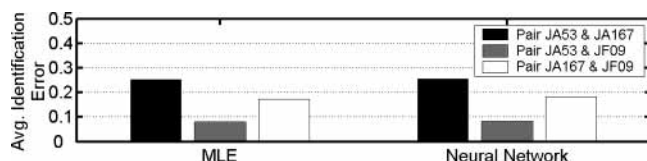
Figure 4. Average identification error for three dye-pairs using MLE and a trained neural network. For each dye tested, there were 1000 training events and 1000 validation events used to train the network. The trained network was evaluated using 2500 test events that were not among those used for training.
